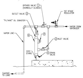
Typical FILTAIRE™ installation shown. Items supplied with standard unit are (4) differential pressure gauges, (5) drain valve, (6) vent, normally plugged. Items (1), (2) and (3) – the bypass valve system for cleaning to be supplied by others at time of installation.
